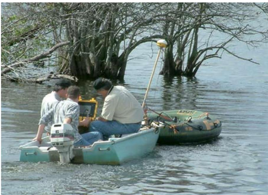
*Making a discharge measurement*
