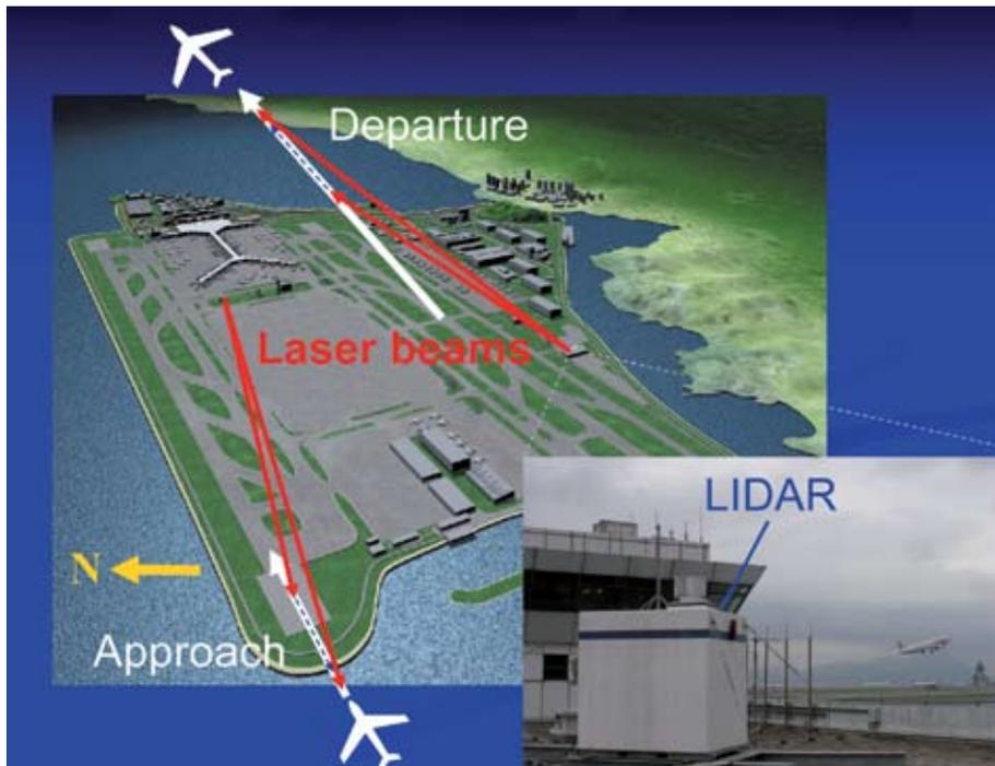
*Schematic diagram of LIDAR wind shear alerting system*
